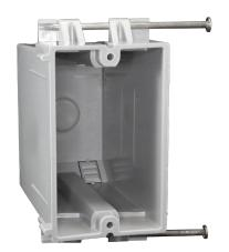
EZ22SN-HW is a 1-gang, 22 cu. in., heavy wall EZ BOX that is ideal for new work applications for residential and light commercial projects where an even more durable box is preferred. The harder shell is designed to resist flexing and hold its shape in extreme conditions. EZ22SN-HW also features enhanced angled nails for easy mounting between studs and knockouts for EZ wiring.
